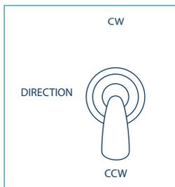
On the rear panel, besides 230V input power connector and the "On-Off switch", you will find the direction switch :
